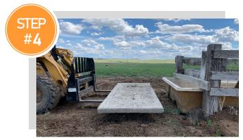
**INSTALL:** Set into place (utilizing the built-in chain system) with a loader and chains, pallet forks, the bale bed on your pickup, or a crane. We recommend filling in any large gaps between the pad and your waterer.
